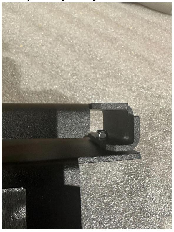
Make sure to position the top panel so that the cutout is on top of the bolt as in the picture below. That is where the factory hard top bolt will be inserted to install your Side MOLLE Panels.
